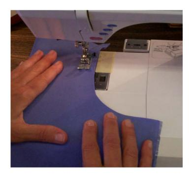
As you sew, guide the fabric, maintaining the curve of the fabric and keeping the fabric flat. Stitching slowly will help a lot, since you'll need to guide the fabric in an arc. The only portion of the fabric that needs to be "straight" is the ½" or so that's directly in front of the presser foot. I like to think of this process as sewing a long, smooth curve.
